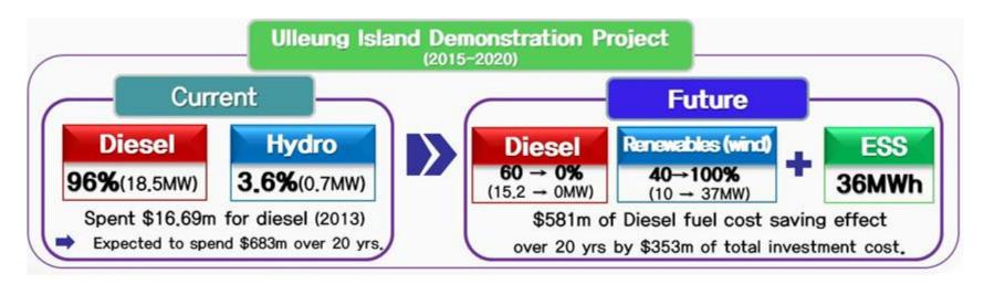
Demonstration is going on in Ulleung Island. Planning to expand a micro-grid model to other off-grid islands in Korea
